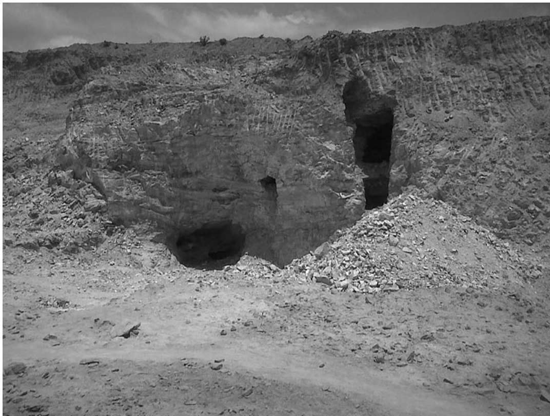
FIGURE 46.1 Shallow undermining into gold-bearing reef. Thousands of these shallow workings exist in the Johannesburg area
